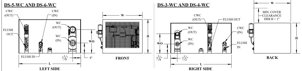
WO: WATER OUTLET WC: WATER CONNECTION SIZE CWC: CITY WATER CONNECTION SIZE
