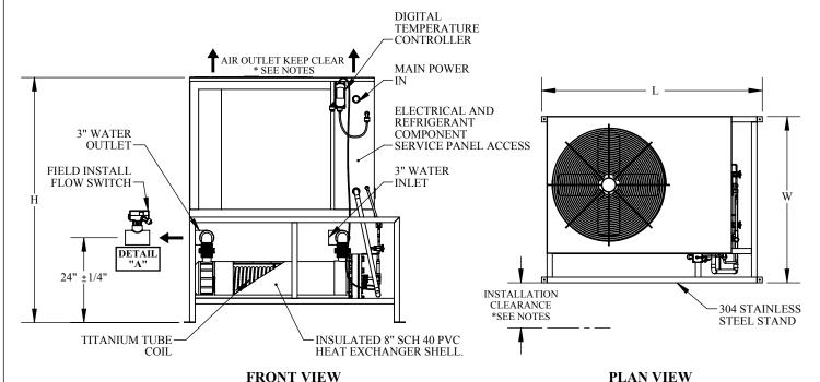
\*INLET, OUTLET AND FLOW SWITCH ARE 3" (SLIP) CONNECTIONS.
